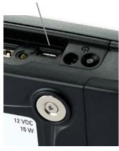
The micro USB port on the DG-1000 can be used to create a wired two-way communication link between the gauge and a Windows computer. Use of the micro USB port requires you to first download and install the appropriate USB Device Driver to the computer using the Windows Update service.
