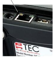
The Ethernet port on the gauge can be used to create a wired two-way communication link with a router or switch (the router or switch must be running DHCP Server).
