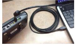
mentioned. After the cable is plugged in the status should change to Connected.
