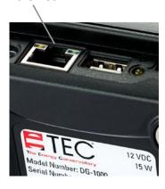
The Ethernet port on the DG-1000 can be used to create a network of gauges that can be used for specialized testing applications, such as big building airtightness testing. Using the gauge's Ethernet port to create a wired multi-gauge network requires a router. A standard
