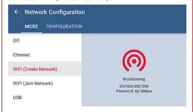
4. The DG-1000 will begin broadcasting a secured wireless network with the following settings
