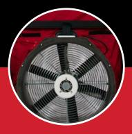
The Minneapolis Blower **Door**™ is used to measure the airtightness of homes and buildings.
