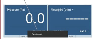
**Note:** The red stop icon will appear on all screens within the Gauge app during cruise, so the fan can be stopped from any screen within the Gauge app. If the Home screen is opened during cruise, the fan will automatically stop.
