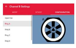
7. Remove the No-Flow Plate from the Blower Door fan and install the flow ring which you think best matches the needed fan flow (see table below.)
