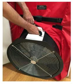
Before conducting the pressurization test, make sure the fan direction is reversed by removing the fan from the nylon panel, and re-inserting it with the exhaust side facing inside the building.
