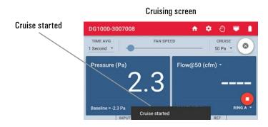
4. The blower door fan will now slowly increase speed until the building depressurization displayed on Channel A is approximately –50 Pa.
