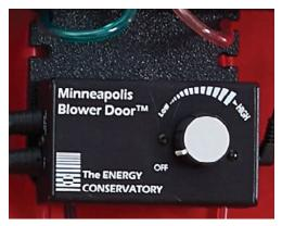
Gradually increase the fan speed by slowly turning the fan controller clockwise. As the fan speed increases, the building depressurization displayed on Channel A should also increase. Continue to increase the fan speed until the building depressurization shown on Channel A is between -45 and -55 Pa.
