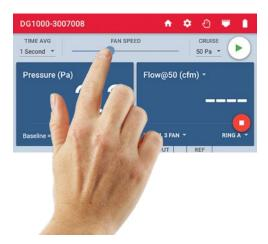
Touch and slide the dot on the fan speed slider in the Gauge app to adjust the fan speed using the DG-1000. As the fan speed increases, the building depressurization displayed on Channel A should also increase. Continue to increase the fan speed until the building depressurization shown on Channel A is between –45 and –55 Pa.
