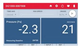
5. During a baseline measurement, Channel A will display a long-term average baseline pressure reading while Channel B is used as a timer in seconds to show the elapsed measurement time. When you are satisfied with the baseline measurement, touch enter and enter the baseline reading into the gauge.
