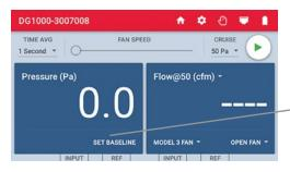
4. With the fan inlet still covered, touch Set Baseline to initiate the building baseline measurement procedure on Channel A.
