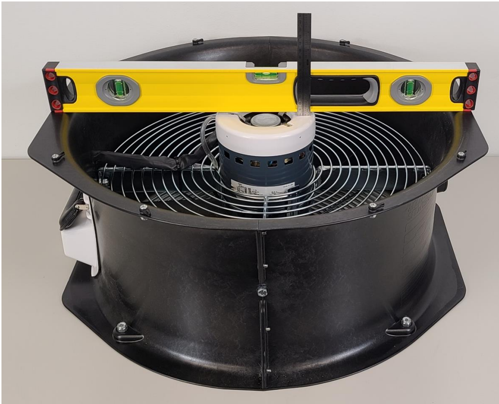
A straightedge across the fan housing with a ruler to measure the gap.
