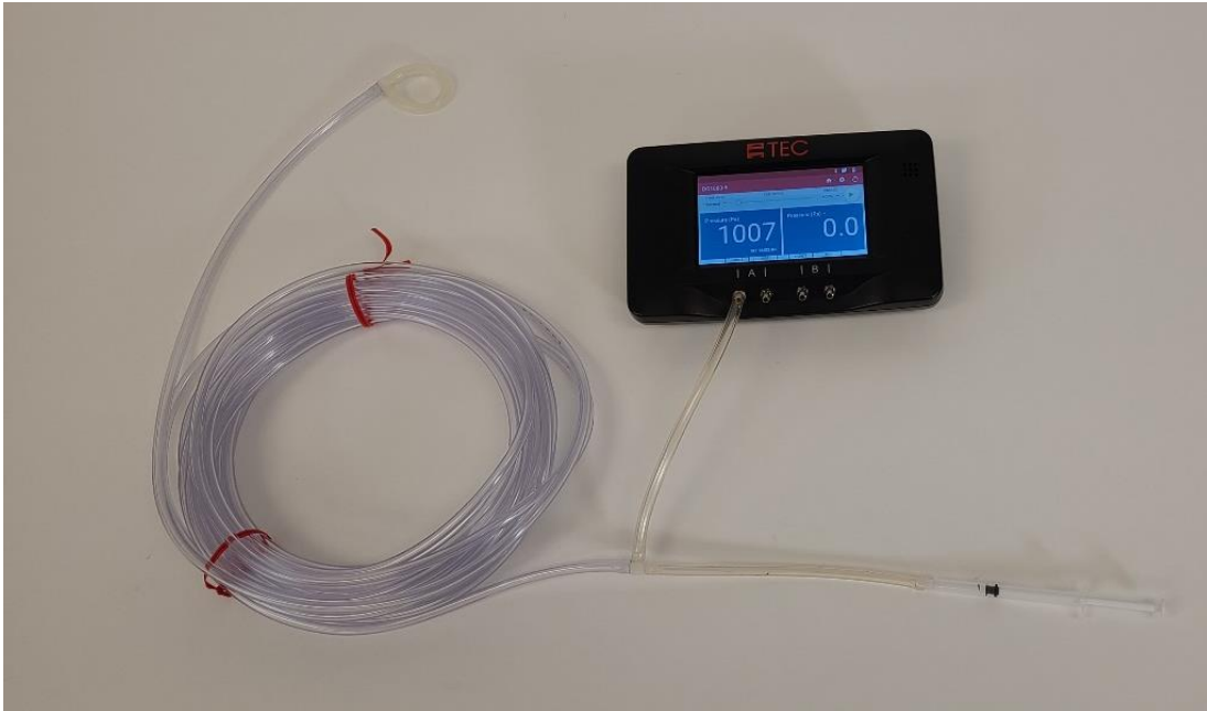
Setup for testing the syringe, tubing, and manometer for leaks.
