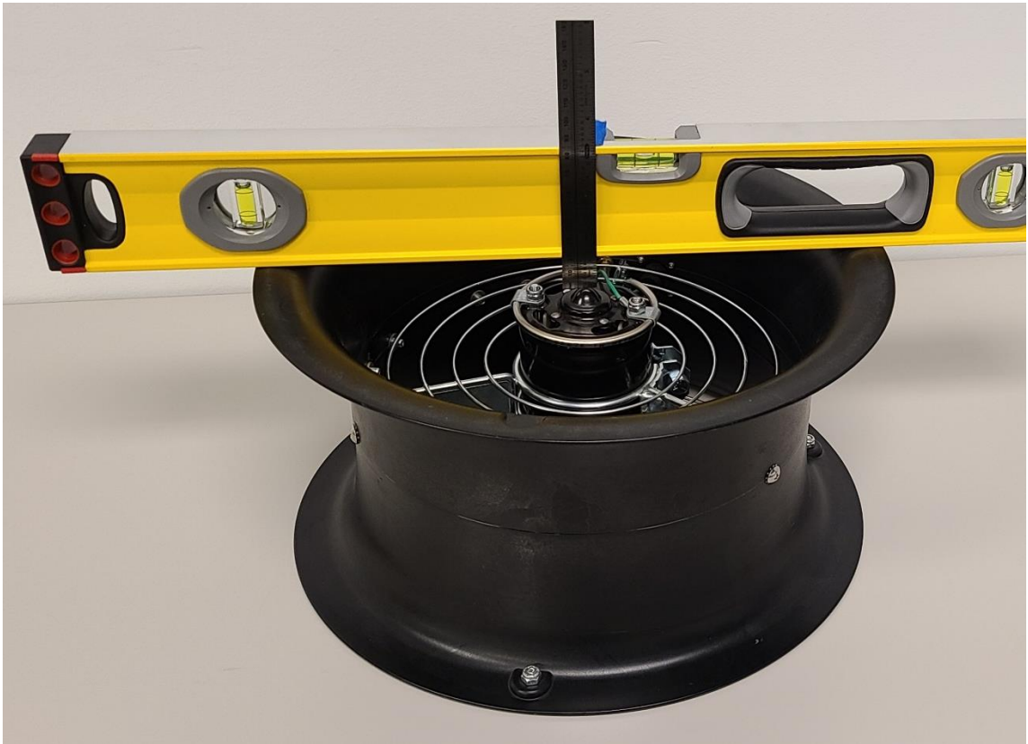
A straightedge across the fan housing with a ruler to measure the gap.
