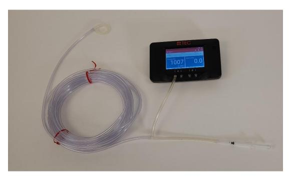
Setup for testing the syringe, tubing, and manometer for leaks.
