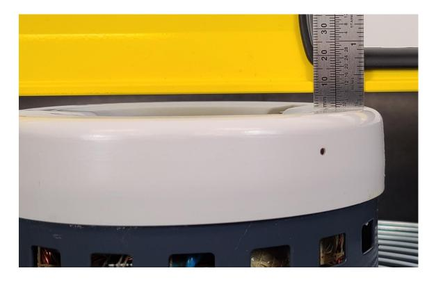
This fan measures just under  $\frac{1}{4}$ " or about 6mm from the flow sensor to the straightedge; it's in the middle of the allowable range.
