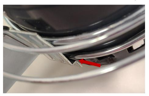
o The same broken weld as seen from inside the housing
