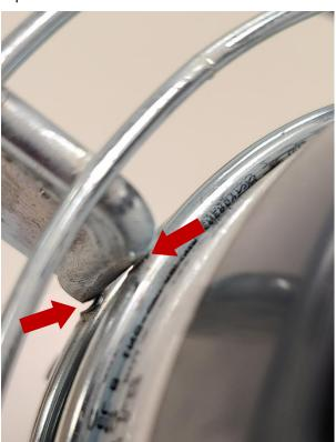
o Broken Between the motor vent tabs and the band clamp
