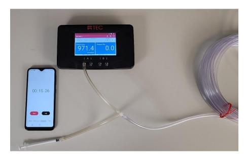
This sensor measures 971 Pa after 15 seconds. It passes the leak test.
