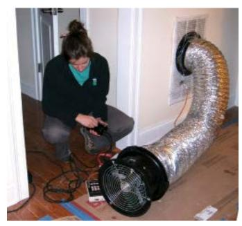
Duct leakage measurements are used to diagnose and demonstrate leakage problems, estimate efficiency losses from duct leakage, and certify the quality of duct system installation.
