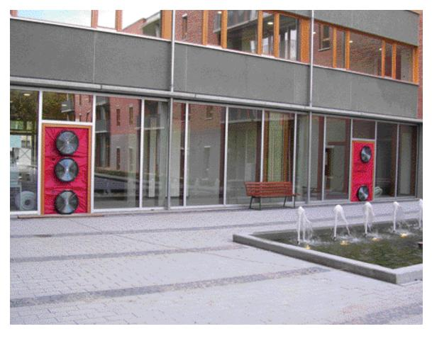
» Air tightness test using two Minneapolis Blower Doors.
