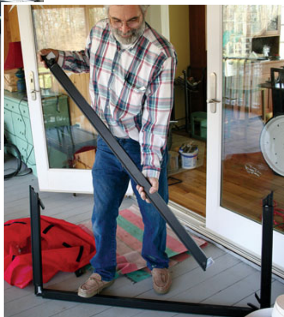
Figure 1. Equipment needed for comprehensive blower-door testing can be packed into a few easily-transported cases (above). The blower door consists of an adjustable aluminum frame and a nylon panel (right), fitted with a powerful variable-speed fan (far right).
