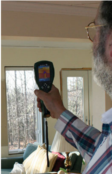
Figure 6. An infrared camera can be a handy tool during a blower-door test. Air leaks around windows and doors typically appear as blue “fingers” on the IR screen, while blue patches (above) indicate conductive losses from problems like thermal bridging, insulation voids, and moisture damage.
