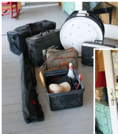
Figure 1. Equipment needed for comprehensive blower-door testing can be packed into a few easily-transported cases (above). The blower door consists of an adjustable aluminum frame and a nylon panel (right), fitted with a powerful variable-speed fan (far right).
