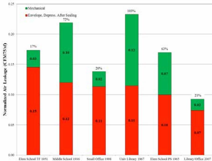
Figure 1 Whole-building leakage tests were conducted with mechanical penetration sealed (red bars) and unsealed. The green bars show the additional leakage due to the mechanical systems.
