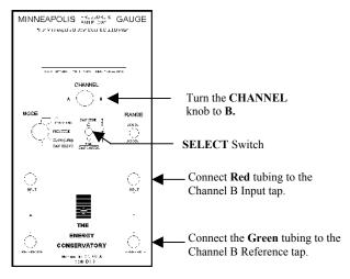
Once the proper plate has been selected, turn the **MODE** switch to *Flow*. With the **CHANNEL** knob set to **B**, the gauge will now display the air flow through the metering plate in CFM. You may want to use the *5 second*, *10 second* or *long-term* time-average setting if the flow reading is fluctuating.
