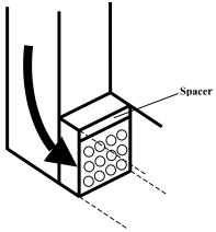
**Note:** If you are installing the metering plate at the filter grille of a single return duct system, simply push the plate into the empty filter rack. Make sure that the front of the metering plate is facing out (into the air flow). Keep the filter grille door open for the remainder of the test.
