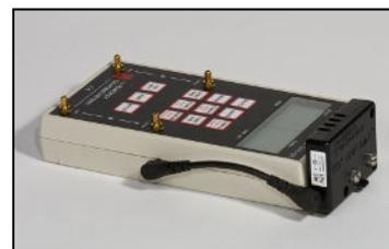
Turn on the DG-700. Once the ON/OFF button is pressed light #2 (green) on the TEC WiFi Link will begin to blink. Light #2 will then turn on solid indicating that it is broadcasting a wireless network access point. The display on the DG-700 should be dashed to indicate that it is ready to be controlled remotely (the keypad is not functional when the display is dashed).
