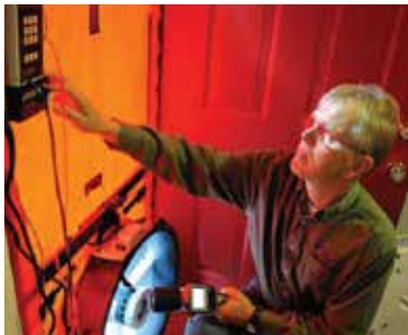
The Minneapolis Blower Door™ airtightness testing system.
