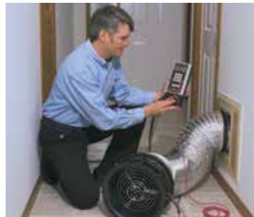
The Minneapolis Duct Blaster® is used to measure the airtightness of ductwork.
