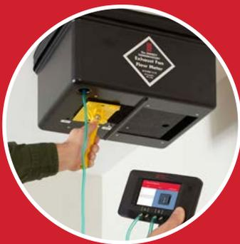
The lightweight Exhaust Fan Flow Meter makes easy work of low flow airflow measurements.
