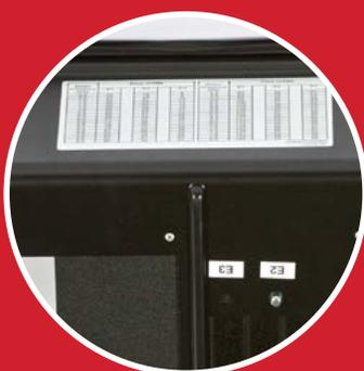
The pressure reading taken from the metering box can easily be converted to air flow using a flow table attached to the side of the metering box.
