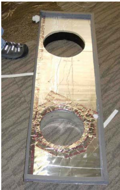
Figure 10: Duct Blaster manifold
