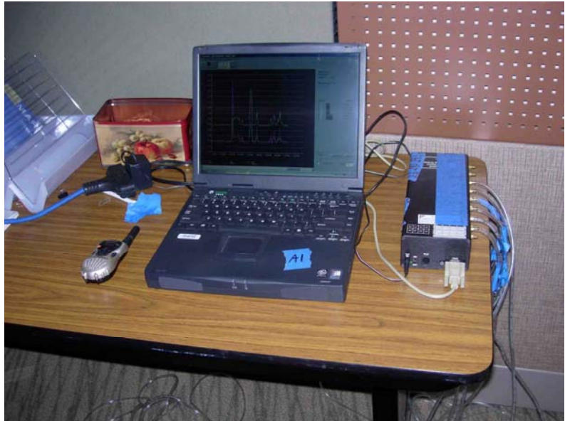
Figure 7: Plenum pressure measurement base station
