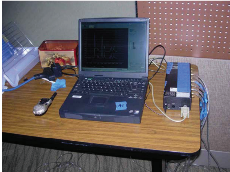
Figure 7: Plenum pressure measurement base station
